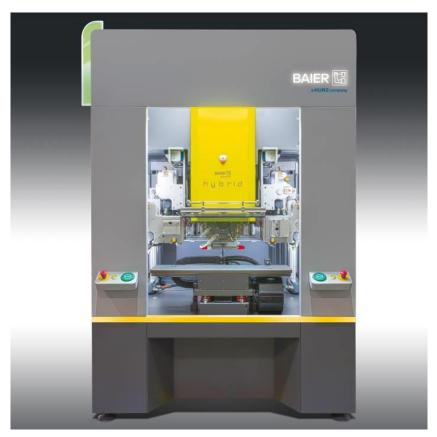
The new Baier hybrid machine for hot stamping decoration and digital printing (Photo: Kurz)
